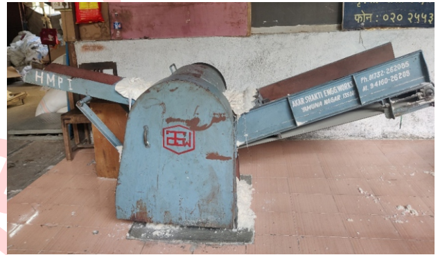
Fig. 3: The shredder machine shreds the fabric and paper waste into a finer form.
