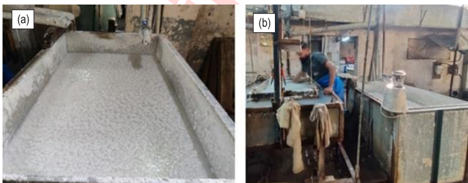
Fig. 6: Paper pulp stored in the tank (a) is used to manufacture paper as shown in (b).
