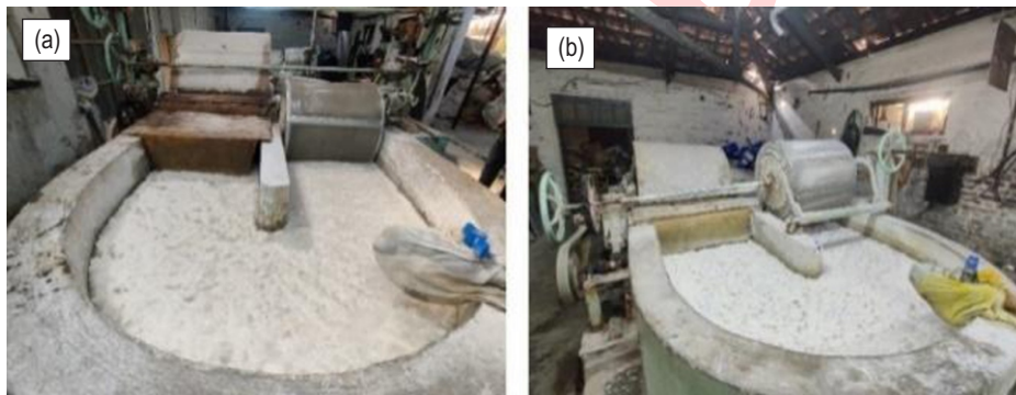
Fig. 5: Pulper machine makes a paste from shredded fabric, along with a combination of paper waste, resin, and dyes.
