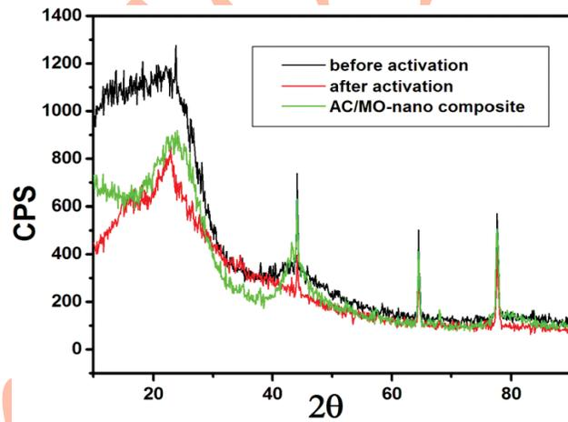
Fig. 3 : XRD patterns of the adsorbents C, AC and composite
