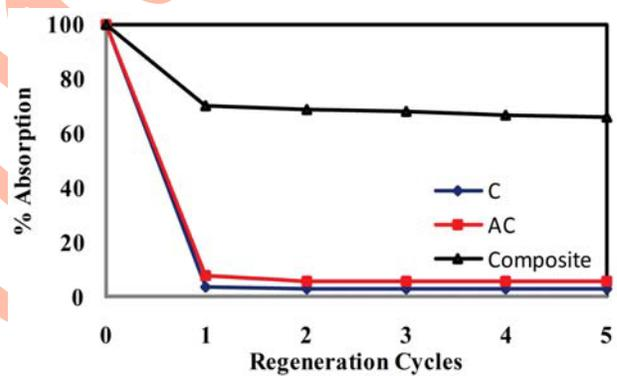
Fig. 8 : Adsorption capability of MB in each of five regeneration cycles with C, AC and Composite
