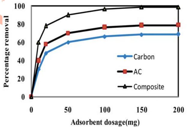
Fig. 5 : Effect of adsorbent dosage on methylene blue adsorbed by C, AC and composite (Adsorbent 100 mg, room temperature 300K and pH 7.0).
