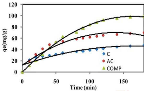
Fig. 7 : Effect of contact time on adsorption capacity of MB adsorbed by C, AC and Composite
