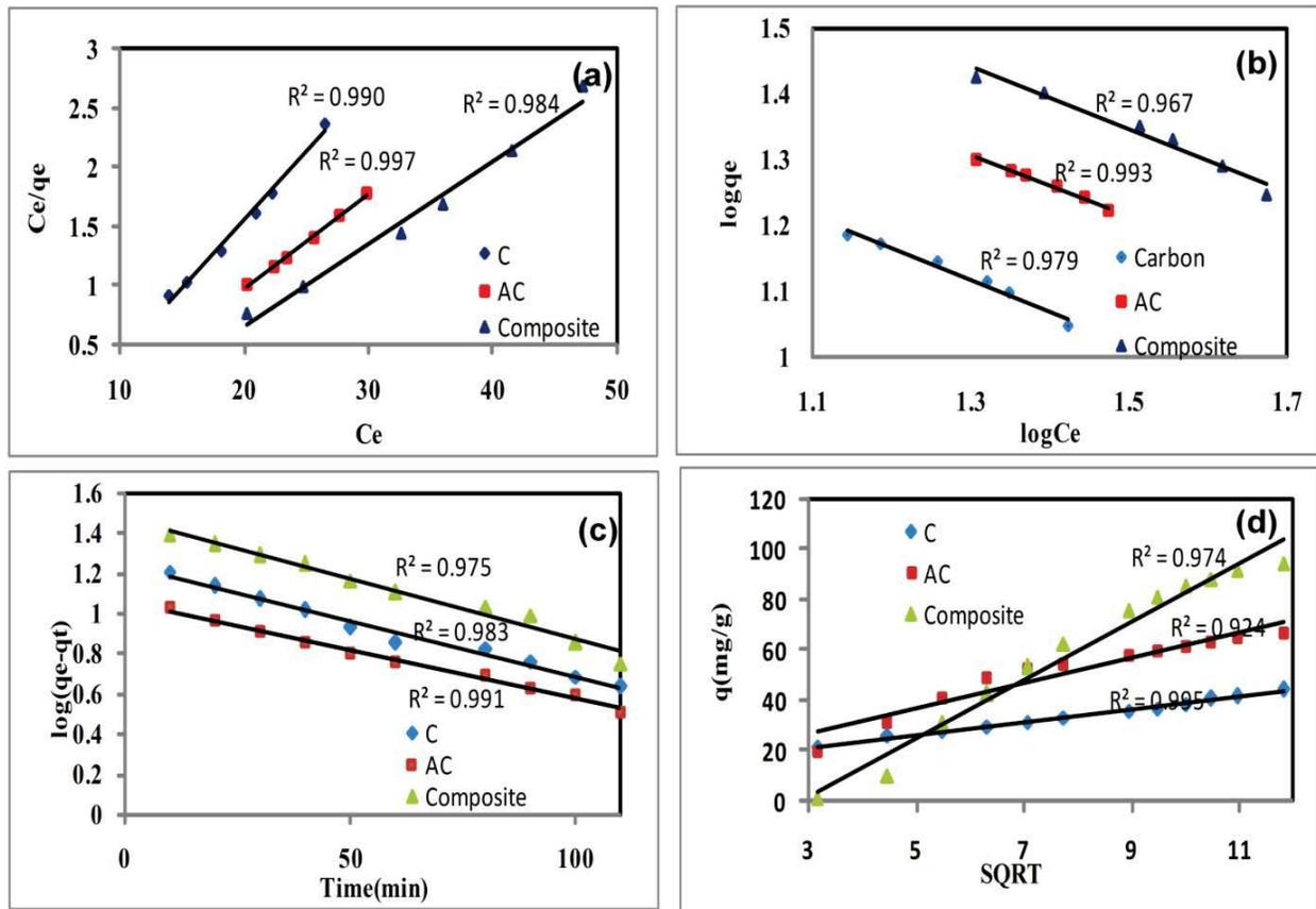
Fig. 6 : Values of methylene blue adsorbed by C, AC and composite by (a) Langmuir isotherm, (b) Freundlich isotherm, (c) Lagergren pseudo first order kinetics isotherm and (d) Intra particle diffusion isotherm
