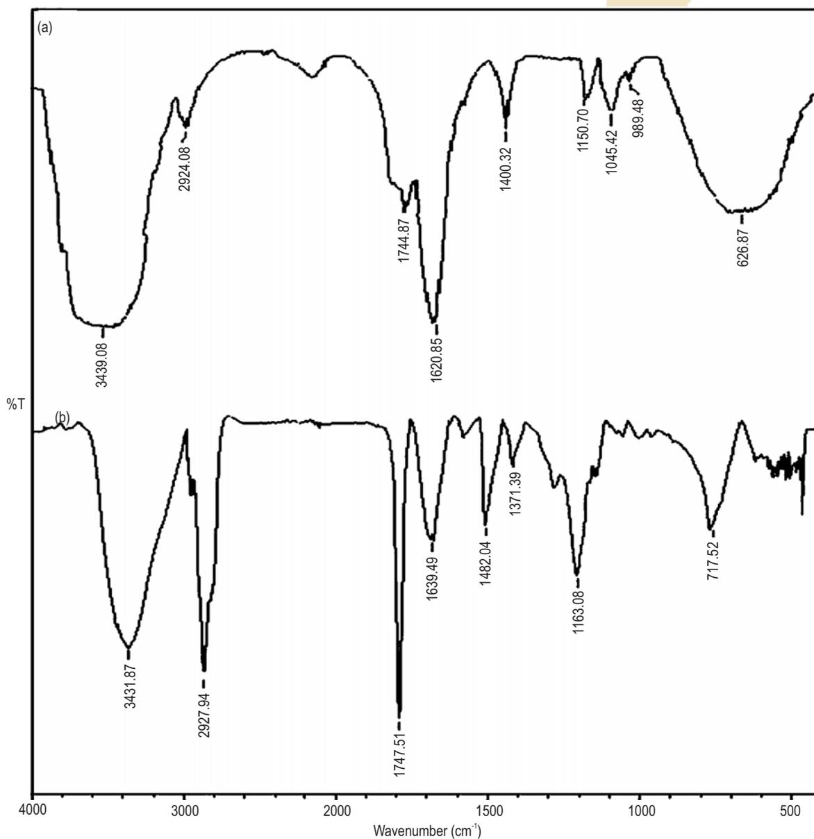
Fig. 2 : FTIR spectra of (a) native biosurfactants and (b) Zn(II) interacted biosurfactant
