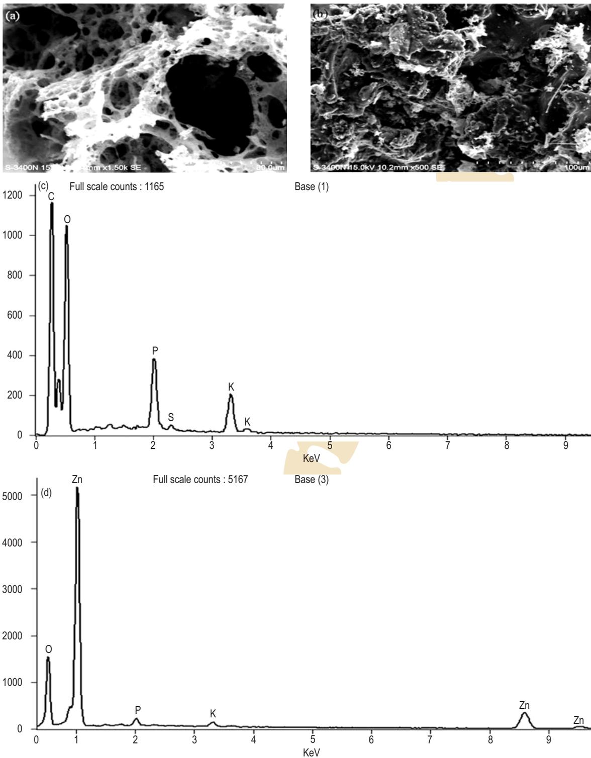
**Fig. 3 :** SEM images of (a) native biosurfactant (b) Zn(II) ions interacted biosurfactant (c) EDS analysis of native biosurfactant (d) Zn(II) ions interacted biosurfactant
