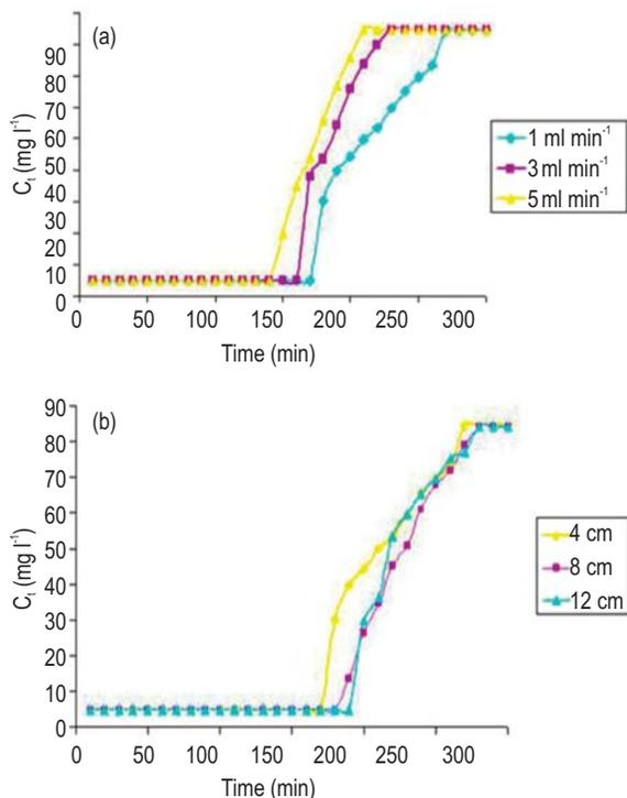
**Fig. 4** Breakthrough curve for Zn(II) removal by biosurfactant (a) different flow rates (b) different bed heights
