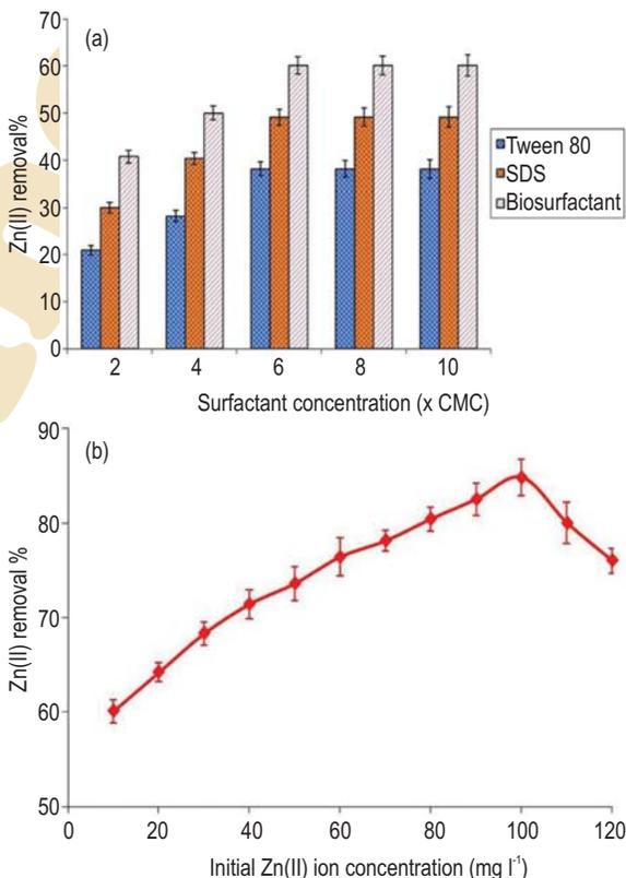
**Fig. 1 :** Percentage of Zn(II) removal (a) at various concentrations by biosurfactant compared with commercial surfactants (b) At various concentrations of Zn(II) ion by 6×CMC of biosurfactant
